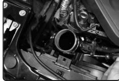
**11.** Tighten the clamp on the turbo side only using 8mm nut driver.
