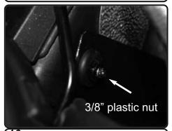
**16.** Secure the tab on heatshield near firewall using the provided 3/8" plastic nut. Secure and tighten.
