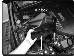
**3.** Now lift up and pull the entire air box out of the vehicle.
