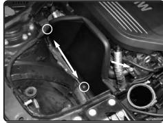
**15.** Push and secure and make sure the grommets are seated and secured to the studs.
