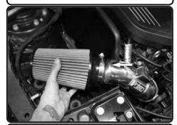
**20.** Install the filter to the intake tube.
