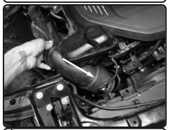
**4.** Loosen the clamp on the turbo using 7mm nut driver and remove the intake tube out of the vehicle.
