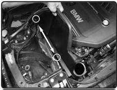
**14.** Install the heatshield into the vehicle and position the 2 grommets to the studs from step 6.
