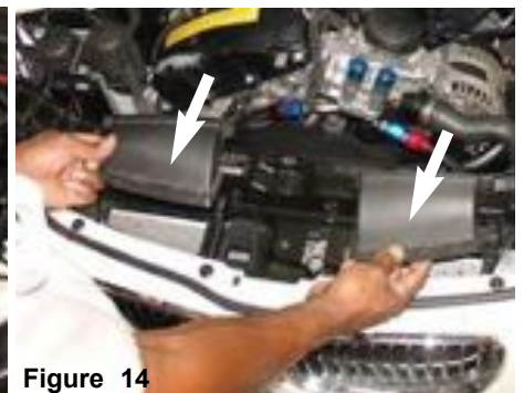
Figure 11 The air box cleaner is now ready to be pulled out of the engine compartment.
