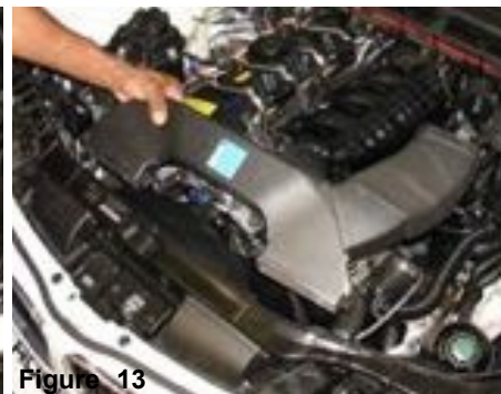
Figure 10 Lift the air box in an up upward motion. Pull the air box grommets away from the two stand-offs located on each side of the runners.
