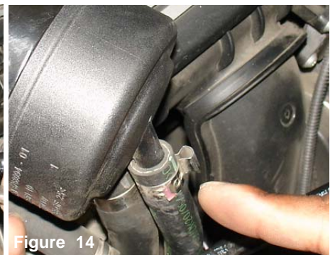
Figure 11 Without disconnecting the two lines, remove the reservoir bottle from the two studs.
