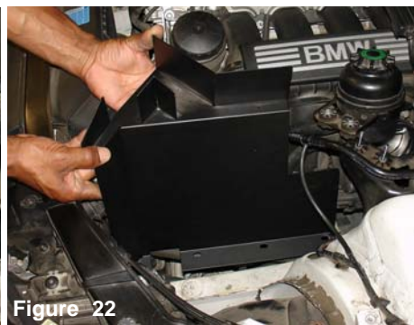
Figure 22 The heat shield is now lowered into the engine compartment.
