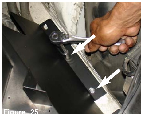
Figure 25 A 10mm socket is used to fasten the flange nuts over the heat shield.
