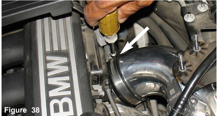
Figure 36 The intake is aligned to the throttle body step hose. Once you have aligned the intake to the step hose, continue to insert the intake into the step hose.
