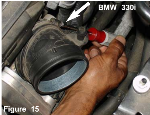
Figure 15 Loosen the throttle body inlet clamp as shown above. The inlet elbow shown above is removed from the 2006 330i
