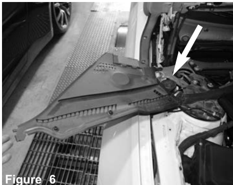
Figure 6 Lift up and turn the engine tray out of the way. This will allow for removal of the factory strut bar. Now repeat and do on other side of vehicle.
