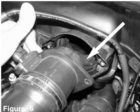
Figure 6 Pull back the MAF sensor housing from the air box.
