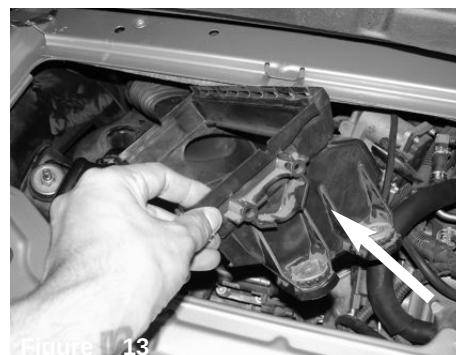
Figure 9 Un-clip the upper half of the stock air box and remove from vehicle.
