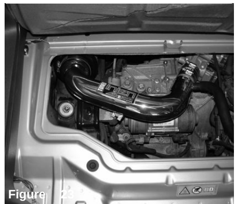
Figure 20 Tighten the clamp on the intake tube using 8mm nut driver.
