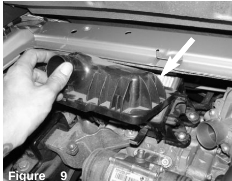
Figure 6 Using a T30 torx bit, loosen the bolt holding in the stock air box located in back of the engine close to the exhaust.
