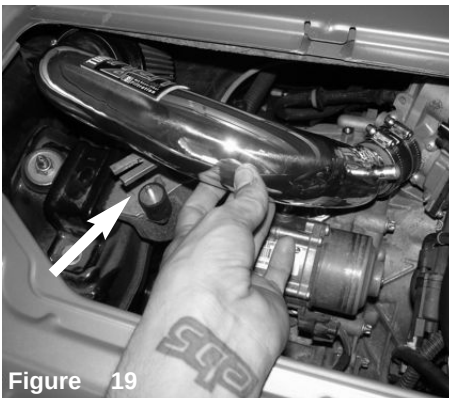
Figure 16 Tighten the clamp on the throttle body using 8mm nut driver.
