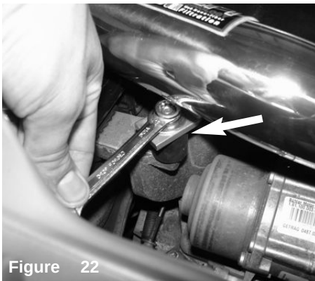
Figure 19 Install the intake system and position the intake tube to the throttle body and bracket to the vibra mount.
