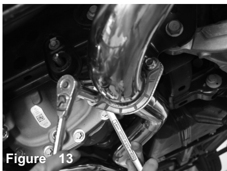
Figure 12 Secure using provided 3" gaskets and bolts with nuts. Do not tighten.
