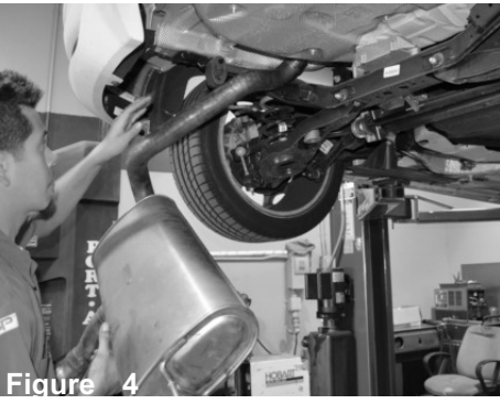
Figure 4 Position the rear muffler section and remove through the frame.
