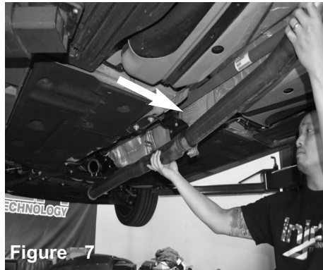
Figure 7 Remove the complete exhaust system out of the vehicle.
