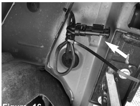
Figure 16 Now with provided Exhaust Valve by-pass module, connect to the harness from step 3. Tighten up and bundle the harness using provided zip-tie. Note: Make sure the Exhaust valve by-pass module is installed or vehicle will not be able to select Drive modes.
