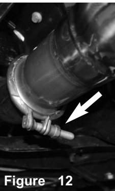
Figure 12 Position exhaust and rotate if necessary. Verify the metal hangar has clearance and does not come close to the drive shaft.
