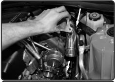
**28.** Now install the last intercooler pipe with turbo flange. Position the 2.5" side to the hump hose. Do not tighten clamp.
