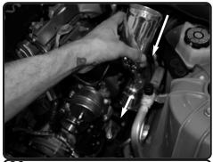
**26.** Install the intercooler pipe with machined fitting side first into same position, This may require to maneuver piping.
