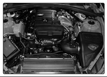
Congratulations! You have just completed the installation of this intercooler pipe system. Periodically, check the alignment of the intercooler pipes, normal wear and tear can cause nuts and bolts to come loose. <u>Note: Check clearance and adjust if needed! Failure to check the alignment and adjust the intercooler pipes can cause damage that will void the warranty. Injen Technology is not responsible for any damages caused by/from improper installation.</u>
