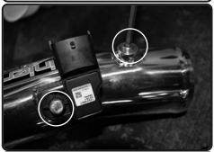
**9.** Install the temperature sensor into the new intercooler tube, secure and tighten using provided M6 screw. If the auxillary NPT fitting is not being used, cap off using provided 1/8" NPT cap.
