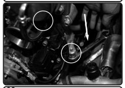
**22.** Loosen the 2 13mm bolts holding in the driverside intercooler pipe flange at the turbo using 13mm wrench.
