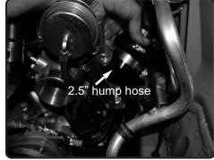
**27.** Once the machined fitting is secured into place, install the provided 2.5" hump hose with clamps provided to the intercooler pipe. Secure on intercooler pipe and tighten clamp.
