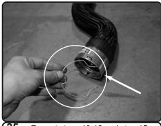
**25.** Repeat steps 10-13 and step 15 for the driver side installation of the intercooler pipe. This will be a 2 piece intercooler pipe.
