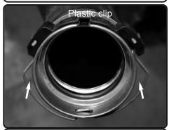
6. Note: the arrows above indicate the where the flathead screwdriver needs to be inserted allowing clip to release from intercooler. The metal clip will lock into plastic clip for release.
