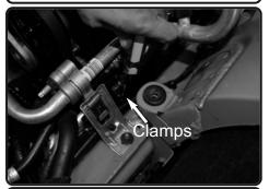
**31.** Secure and tighten clamps using 8mm nut driver. Re-install guard, and intake system. Your intercooler pipe kit is now complete.
