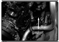
**29.** Position the flange to the turbo. Install the gasket from step 23. Secure using original 13mm bolts.
