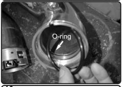
**10.** Install the provided o-ring to the machined fitting. locate the groove cut out and install.
