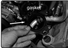
**23.** Save the gasket and bolts for later use. Keep the gasket when installed in same direction.
