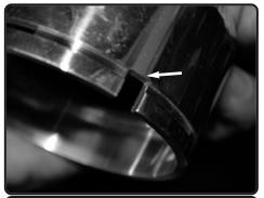
15. Make sure the cut out for lock is seated properly. make sure you hear the click of the metal clip and pull back to verify its secured properly.
