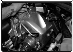
**20.** Remove the exhaust manifold cover using 10mm socket or wrench.
