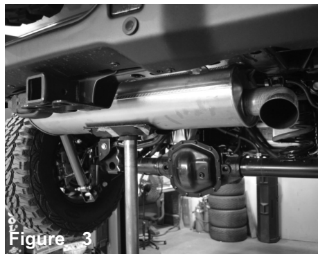
OEM exhaust system. Secure vehicle on lift. Loosen the 15mm nut on OEM clamp. Loosen and pull back.
