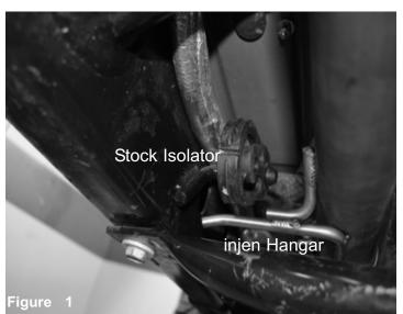
Remove the stock muffler using 15mm socket and wrench. Remove the hangars from stock isolators. Install the new Injen High Tuck Exhaust. Position the hangars to the stock isolators. (you wil only use 2 factory isolators in the kit.) Use Provided #63 torsion clamp in the kit. Position for the best to have access to the 17mm nut on clamp. Make sure the flared section on exhaust installs to the factory unit and bottoms out and stops. *Do not tighten*.
