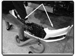
7. Remove the front bumper cover, remove screws on top and bottom. Carefully pop out. Disconnect the camera and sensors also.
