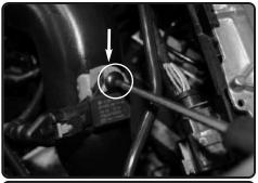
**11.** Loosen the sensor using T25 torx bit.
