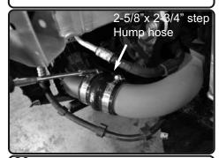
**20.** Install the 2-5/8" x 2-3/4" step hump hose with clamps to the intercooler and connect. adjust for clearance and fitment.
