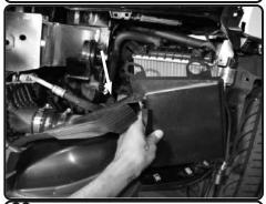
**22.** Secure and re-tighten the horn bracket and trans cooler. Re-install the trans cooler cover. Re-install bumper cover and re-connect sensors and camera.
