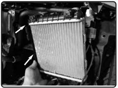
**15.** Loosen the trans cooler bracket and pull back. this will allow for installation of the injen cold side intercooler tube.
