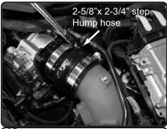
**18.** Install the provided 2-5/8" x 2-3/4" step hump hose with clamps to the throttle body. Do not tighten
