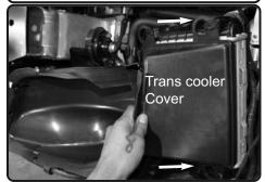
**8.** Slide the trans cooler cover over and remove.
