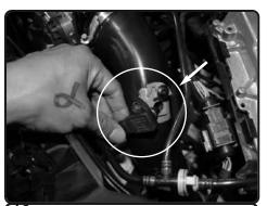
**12.** Now push the clip down and rotate the sensor out of the intercooler tube.
