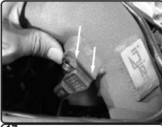
**17.** Install the temperature sensor to the machined pad and secure using provided M5 hex screw. Tighten using 8mm nut driver.
