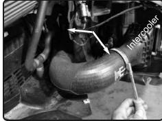
**3.** Once the bumper is removed. Start by loosening the hot side intercooler OEM rubber hose using 7mm nut driver on both sides.
