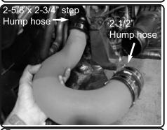
**5.** Install the injen hot side intercooler pipe using the 2-5/8"x 2-3/4" step hump hose and 2-1/2" hump hose with clamps provided.
