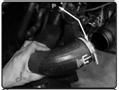
**4.** Once both sides are loosend, carefully remove the OEM hose out of vehicle.
