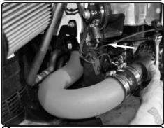
**6.** Adjust for fitment and tighten clamps using 8mm nut driver or ratchet.
