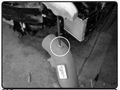
**16.** Install the provided 1/8" NPT plug to the fitting on the intake tube. secure and tighten using allen key. Install intercooler tube into the vehicle from bottom up and position.
