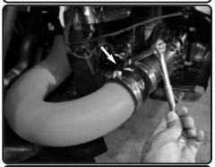
**7.** Verify the clamps are tightend and secured.
