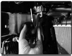
**14.** Loosen the horn bracket and pull back.
