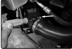
**9.** Once removed, loosen the clamp on the cold side of the intercooler pipe using 7mm nut driver.
