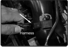
**10.** Disconnect the Temperature sensor harness.
