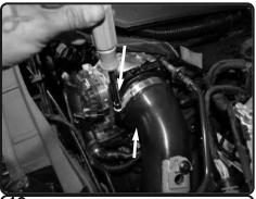
**13.** Loosen the clamp on the throttle body using 7mm nut driver. Pull out and remove from the vehicle from down under the vehicle
