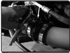
**21.** Secure and tighten all clamps using 8mm nut driver or ratchet.
