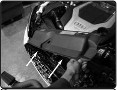
**2.** Push clip on hood release lever, and remove. Lift up and pull back the grille cover.
