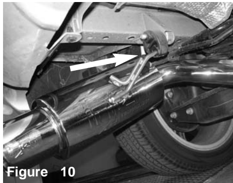
Figure 10 Install the exhaust sytem and position hanger to the rubber hanger.
