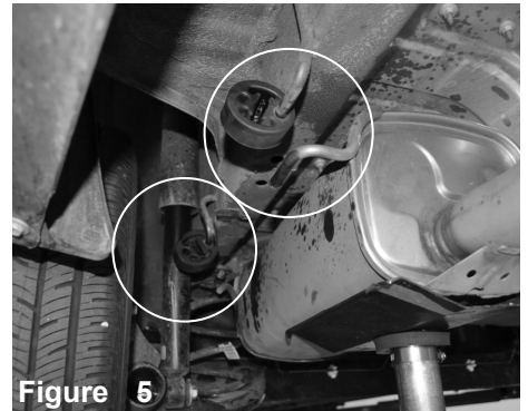
With lubrication, loosen and remove the 3 rubber isolators and remove the rear section of the exhaust.
