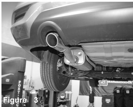
OEM exhaust system. Secure vehicle on lift.
