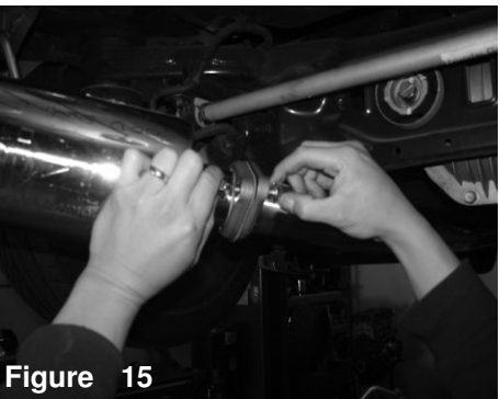
Figure 12 Install the driver side rear section and position the injen exhaust rear hanger to rubber hanger.
