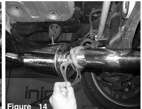
Figure 14 Install the flange and connect the two together.
