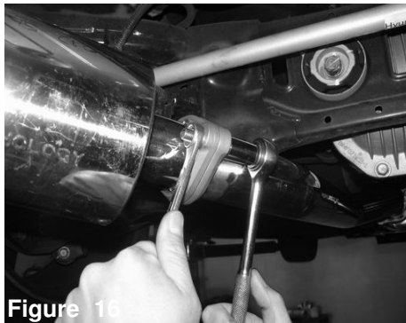
Figure 13 Secure the two parts using provided M10 bolts and nuts. DO NOT TIGHTEN!
