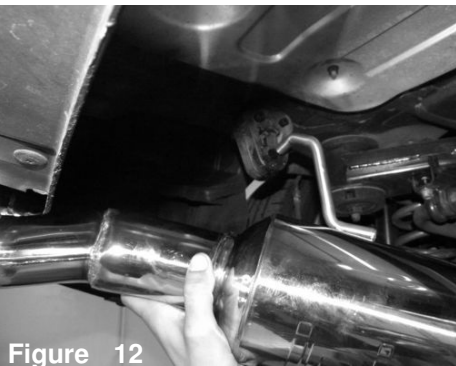
Figure 12 Install the driver side rear section and position the injen exhaust rear hanger to rubber hanger.
