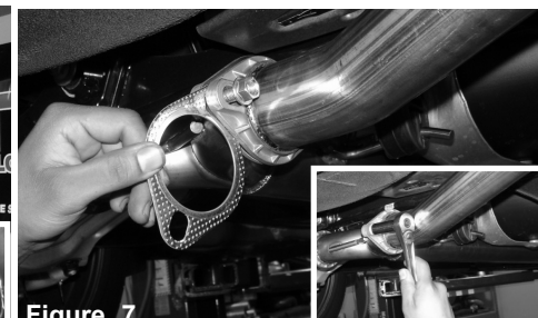
Figure 7 Place one supplied 60mm gasket and two M10 nuts and bolts connecting the right side muffler section flange to the mid-pipe flange. Use a 14mm ratchet and socket to snug the two M14 nuts and bolts for now. Do not tighten them. Repeat this process for the left side muffler section.
