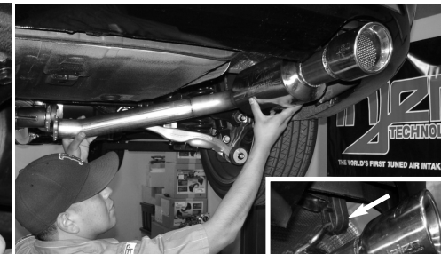
Figure 6 Once the mid-pipe is in place. Position the right side muffler section into the right side bumper cavity and then hang the muffler on the grommet.
