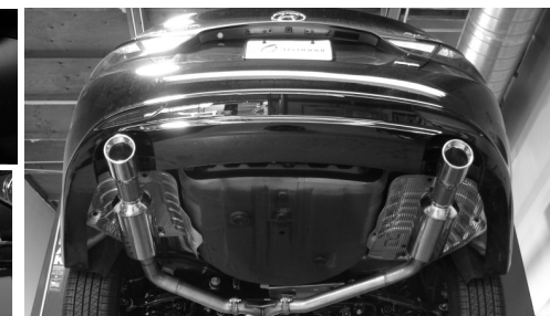
Figure 8 Make sure nothing comes into contact with any component and then make your final adjustments to the entire exhaust system. Use a 14mm socket and ratchet secure all the M10 nuts and bolts. Congratulations! You have just completed the installation of the Injen Cat-back system. Periodically, check the alignment of the exhaust, normal heat cycles can cause nuts and bolts to come loose. Failure to check the alignment and adjust the exhaust can cause damage that will void the warranty.
