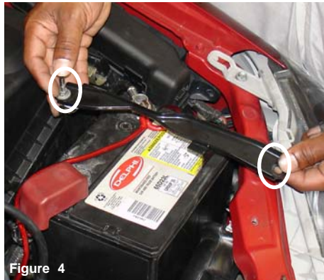
Figure 4 Loosen and remove the two m6 nuts from the battery tie down braces as shown above. Disconnect and remove the battery cables from the battery post.
