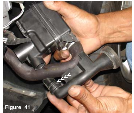
Figure 41 The resonator box and spout is now removed and the spout will be separated from the box as shown above.
