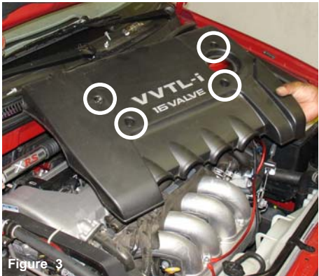
Figure 3 Loosen and remove all four m6 nuts holding the engine cover in place.
