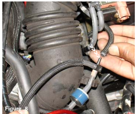
Figure 8 Disconnect the vacuum switching valve line that is connected to the one way check valve.
