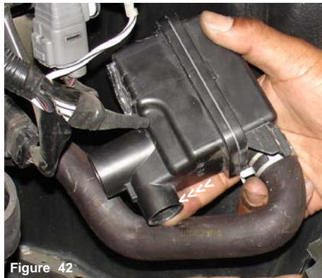
Figure 42 The connecting spout between the lower resonator box and the upper resonator box has been removed from the port shown above.
