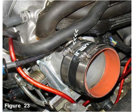
Figure 23 Press the 2 3/4" straight hose over the throttle body, use two power-bands on the hose. Tighten the clamp on the throttle body side for now.
