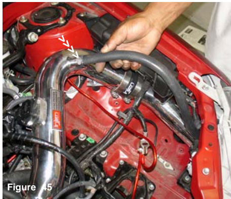
Figure 42 The connecting spout between the lower resonator box and the upper resonator box has been removed from the port shown above.
