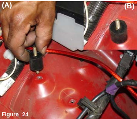
Figure 24 Align the vibra-mount to the pre-tapped hole on the strut tower mount (A). The vibra-mount is now sitting flush on the strut tower mount (B).
