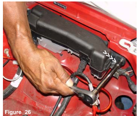
Figure 26 Loosen and remove the m6 bolt on the fuse box located on the fender wall.
