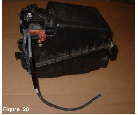
Figure 20 The assembled air box cleaner that has been removed from the engine compartment including the VAD vacuum switching valve, which is no longer used
