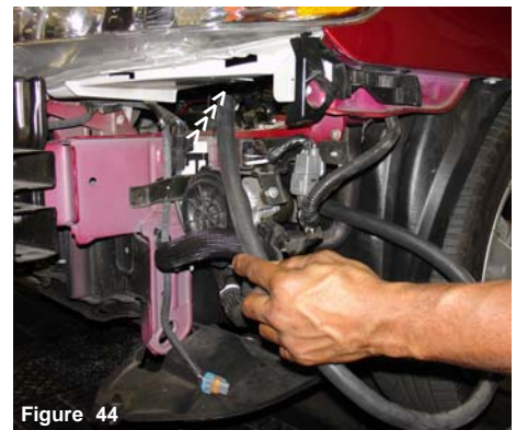
Figure 44 The remaining 17mm hose is placed under the head lamp and inserted into the engine compartment.
