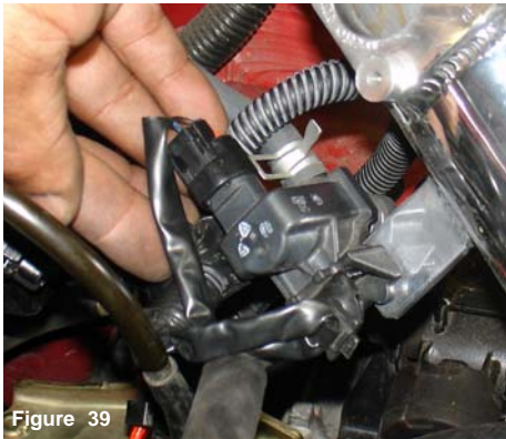
Figure 39 The PWM vacuum switching valve is now installed.
