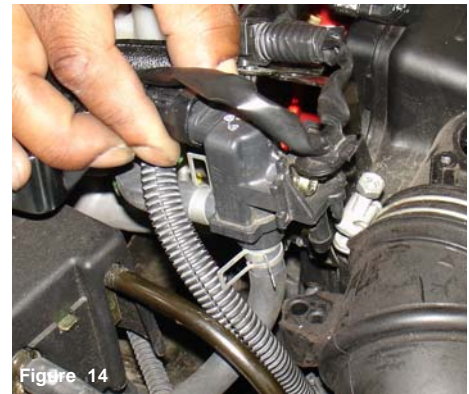
Figure 11 Once you have removed the two screws, continue to remove the mass air flow sensor from the sensor housing.
