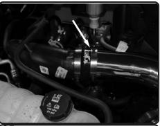
**25.** Tighten clamp using 8mm nut driver.
