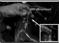
**21.** Install the vibramount to the welded fitting on intake tube, secure the vibramount and tighten.
