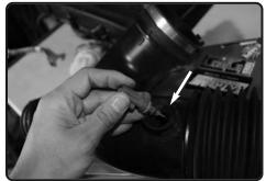
**8.** Loosen and remove the temperature sensor out of stock intake. Use a small flat head screwdriver to pull back clip on sensor.
