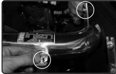
**23.** Secure the brackets using provided M6 nuts and fender washers.
