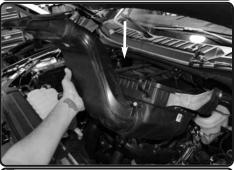
7. Now lift up and remove the bottom half of air box out of vehicle.
