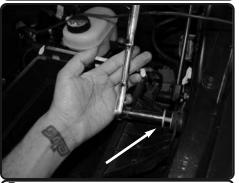
**5.** Loosen the bolt holding in the bottom of the airbox using 13mm socket or wrench.
