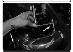
**20.** Secure the bracket using provided m6 nut and fender washer tighten using 10mm socket and ratchet. Tighten clamps using 8mm nut driver.
