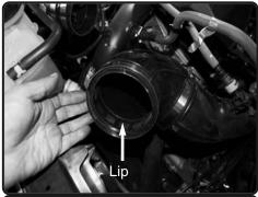
**16.** Now install the 4" elbow with clamps provided to the large turbo housing side. Make sure the side with no lip is installed on the housing. Position like image above.
