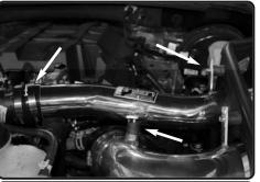
**22.** Now install the smaller intake tube. Position tube to 3" hose and brackets to vibramounts.
