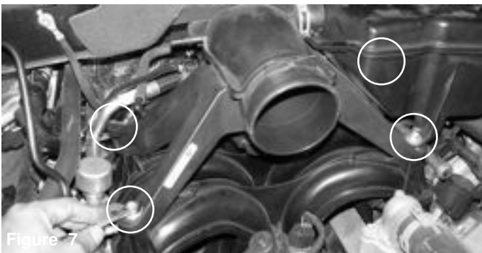
Figure 5 Un-clip the 3 clips holding in upper half of air box and slide back.
