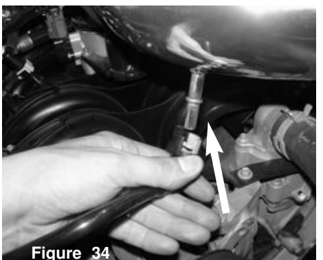
Figure 31 Now tighten the clamps on throttle body using 8mm nut driver.
