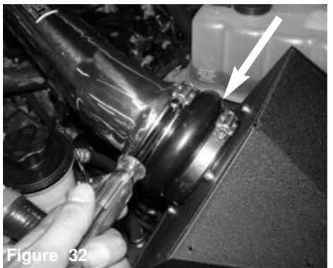
Figure 29 Install the intake tube into the vehicle and position to the throttle body and adaptor.
