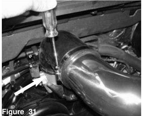
Figure 31 Now tighten the clamps on throttle body using 8mm nut driver.
