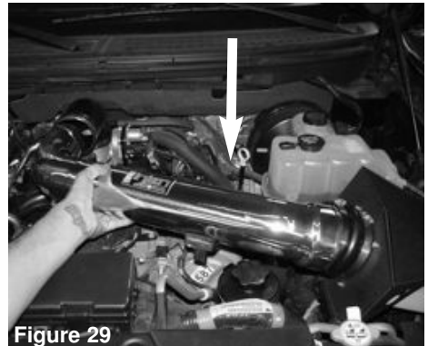
Figure 29 Install the intake tube into the vehicle and position to the throttle body and adaptor.
