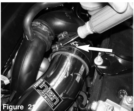
Figure 22 Reconnect the temp sensor harness.
