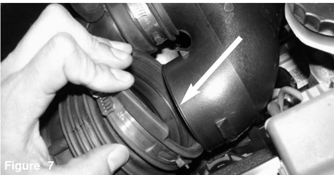
Figure 5 Loosen the intake tube clamp using 8mm nut driver.
