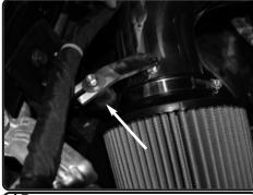
**15.** Secure the bracket using provided M6 nut and fender washer.
