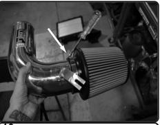
13. Install the filter to the intake tube and tighten using 8mm nut driver.
