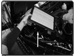
**4.** Lift up and remove the lower part of the air box assembly.
