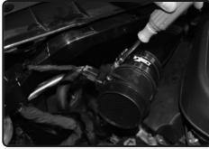
**11.** Rotate the MAF sensor and connect the harness. Tighten clamp on MAF sensor.
