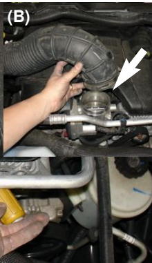
Figure 7(A) Use a 8mm nut driver and loosen clamp on air duct connected to throttlebody.
