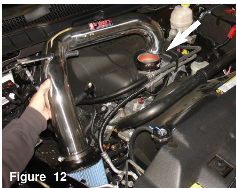
Figure 13 Position the intake pipe into the engine bay and line up the end of the pipe into the throttlebody.
