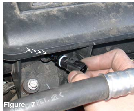
Figure 4 Disconnect the electrical harness clip from the air temperature sensor (A). The m8 bolt is also removed from the intake resonator top (B).
