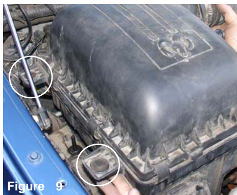
Figure 6 The second m8 bolt is removed from the air intake resonator located just above the oil cap.
