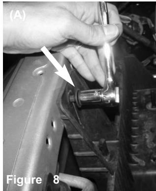
Figure 8 (A) Loosen the bolt holding in the air box plastic bracket closes to the headlight. (B) Remove the bolt and save for the bracket install.
