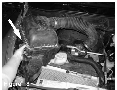
Figure 8 Lift factory air box cleaner and pull entire air box and air duct assembly out of engine bay.
