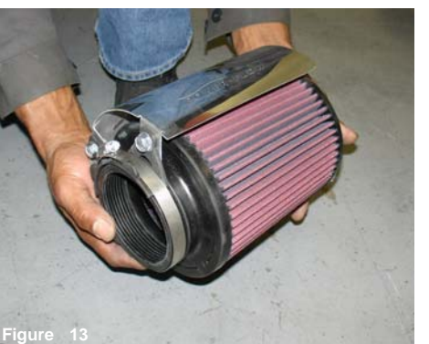
Figure 13 Filter and heat shield assembly is now complete.
