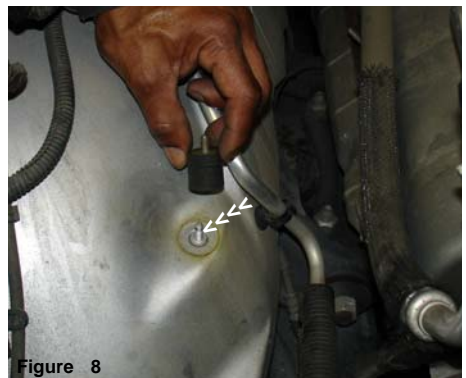
Figure 8 Align and screw the vibra-mount into the m6 stud located over the wheel well.
