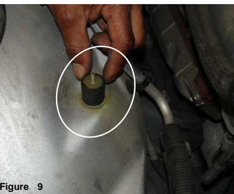
Figure 9 The male/female vibra-mount is now sitting flush with the wheel well.
