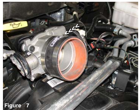
Figure 7 Press the 3/4" straight hose over the throttle body. Place two power bands over the straight hose, tighten the clamp located over the throttle body side.
