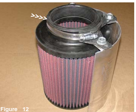
Figure 12 Adjust the clamp so that it sit between the filter beads located on the filter neck.
