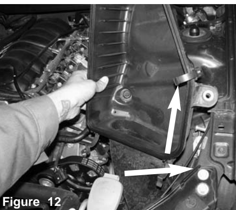
Figure 9 Un-clip the upper half of air box and remove.
