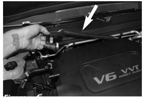
Figure 4 Pull the crankcase line from the back of the engine cover/airbox.
