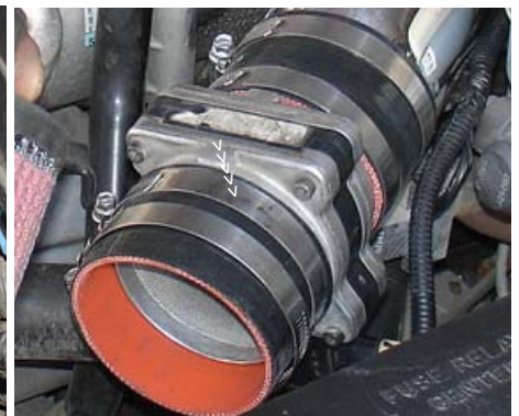
Press the remaining 3 1/4" straight hose over the end of the mass air flow sensor. Place two power-clamps on the sensor and tighten the clamp on the sensor side.
