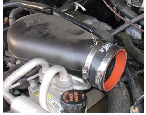
The 3 1/2" straight hose is pressed over the plastic air inlet elbow and two clamps are used. Tighten the clamp that is located on the elbow.
