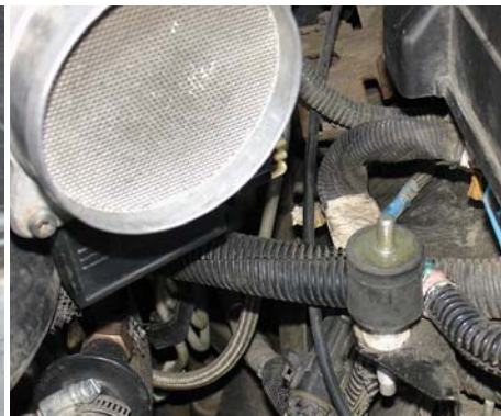
Screw the vibra-mount into the stud until it sit flush and firm.
