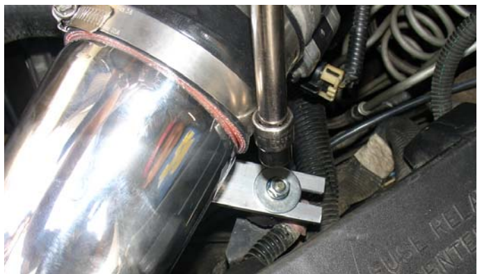
Use the m6 flange nut and fender washer to fasten the intake bracket to the vibra-mount stud.
