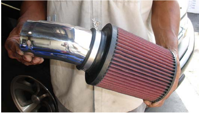
Press the 3 1/2" inverted filter over the end of the secondary intake. Press the intake into the filter until it butts up against the filter stops. Once the filter and the intake have been butted up continue to tighten the filter neck clamp.
