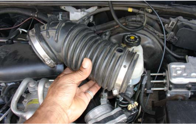
Disconnect and remove the air intake duct between the throttle body air inlet and the mass air flow sensor.
