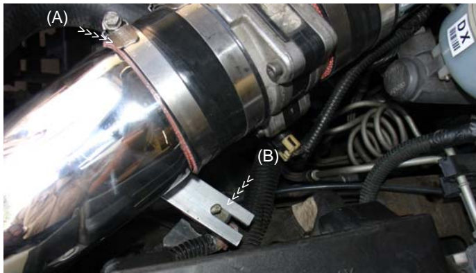
The secondary intake is pressed into the 3 1/4" hose located on the air mass sensor (A) while the intake bracket is lined up to the vibra-mount stud (B).
