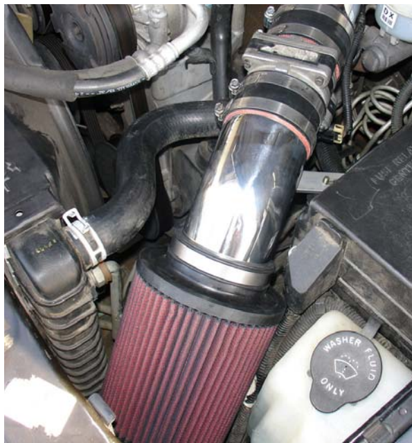
Align the entire intake for the best possible fit. Once the intake has been cleared from rubbing or moving parts continue to tighten all nuts, bolts and clamps.
