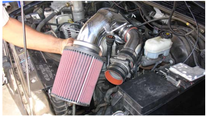
Place the assembled intake and filter into the engine compartment and align the intake to the mass air flow sensor. The intake bracket will also be aligned to the vibra-mount stud.
