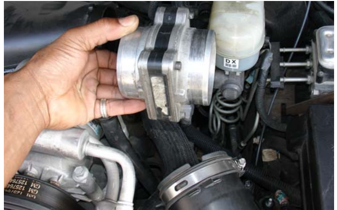
Loosen the last clamp and remove the mass air flow sensors shown above.
