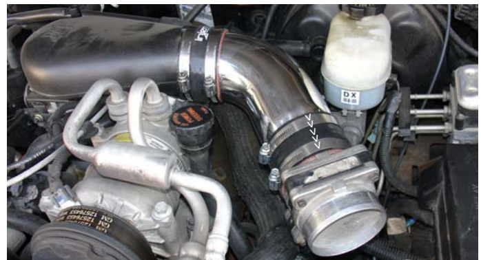
Press the mass air flow sensor into the end of the 3 1/4" straight hose as shown above, semi-tighten the clamp for now.
