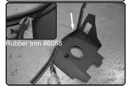
**8.** Now install the rubber trim to the top of heat shield. Notch corners with cutters or pliers for easier installation.
