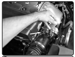
7. With 8mm nut driver, loosen the clamp on the throttle body and pull back tube from turbo.
