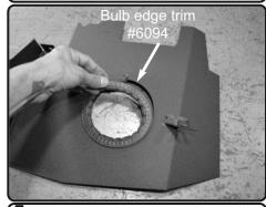
**7.** Install the provided Bulb edge trim to the hole cut out on heatshield. (If trim is long, cut to length)
