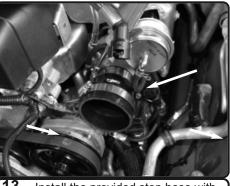
**13.** Install the provided step hose with clamps provided to the turbo. Tighten clamp on turbo only using 8mm nut driver.
