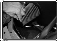
**22.** Check with clearance, and adjust the intake tube. Make sure filter top does not hit frame and fender splash guard.
