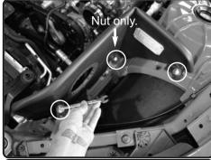
**15.** Secure the heatshied using provided fender washers and M6 nuts. Bracket in back corner will only have nut, no fender washer.
