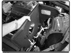
**14.** Now install the heatshield into the vehicle. Position the brackets on heat shield to the vibramounts.
