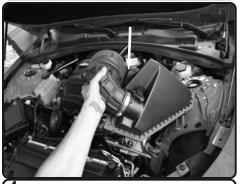
**4.** Now Lift up air box from vehicle and remove complete stock air box assembly.
