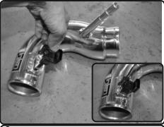
**6.** Now install the MAF sensor into the injen intake tube. Secure using provided M4 button head screws and tighten using 2.5mm allen key.
