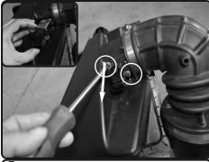
**5.** With t25 torx bit, loosen and remove the 2 screws holding in the MAF sensor.
