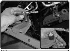
11. Now install the 3 provided vibramounts to the same holes where grommets were just removed. Center the vibramount to hole. Secure the vibramounts using provided washer and nut.
