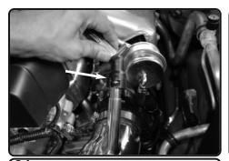
**24.** Re-connect the Crank case line to the fitting on intake tube. *Make sure you hear the click*
