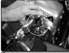
Now disconnect the Crank case fitting from the intake tube and pull back from tube.
