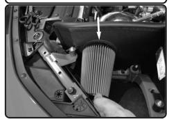
**20.** Install the filter and position to intake tube.
