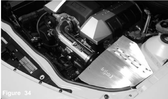
Figure 32 Secure cover using M6 button head screws and tighten using 4mm allen key.
