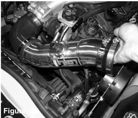
Figure 25 Install MAF sensor to intake tube.
