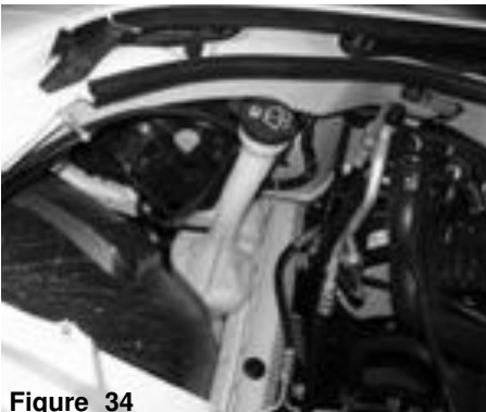
Top view of the reservoir bottle spout after the air box cleaner has been removed.
