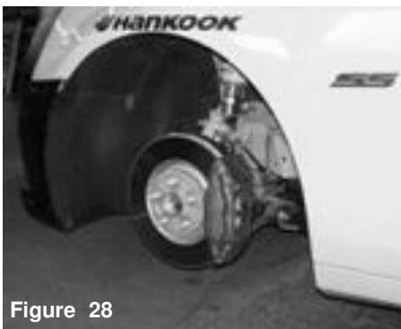
The wheel is now pulled-off as shown above.
