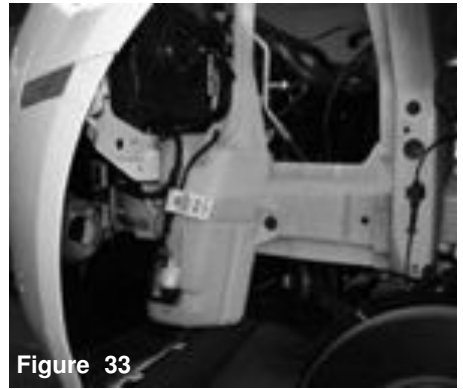
Side view of the reservoir bottle after the wheel and splash guard have been removed.
