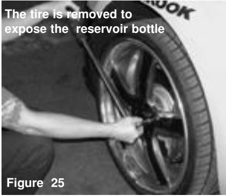
The tire is removed to expose the reservoir bottle
