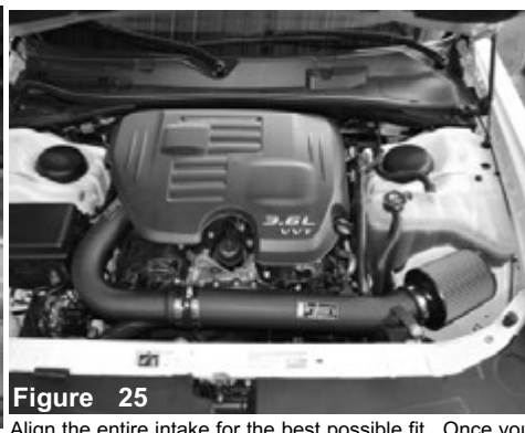
Figure 25 Align the entire intake for the best possible fit. Once you have rechecked and cleared the intake from all moving parts, continue to tighten all nuts, bolts and clamps.
