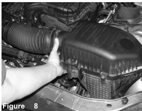
Figure 8 Now lift up and remove the complete stock air box assembly
