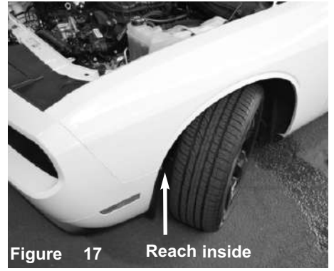
Figure 17: Reach inside. Turn the steering wheel to the left. This will give you access to the outer wheel well to secure the M6 nut to the vibramount from figure 16. No wrench necessary, just turn the vibramount until it's snug.
