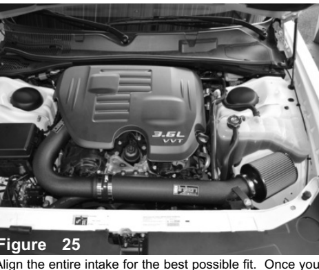
Figure 25 Align the entire intake for the best possible fit. Once you have rechecked and cleared the intake from all moving parts, continue to tighten all nuts, bolts and clamps.
