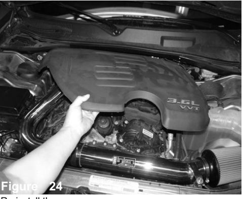
Figure 24 Re-install the cover.
