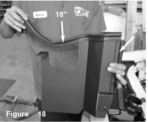
Figure 18 Place the 8" vinyl trim onto the right side of the heatshield and the 18" vinyl trim onto the top side.
