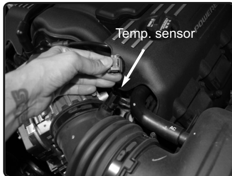
2. Disconnect the Temperature sensor harness.
