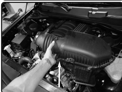
5. Carefully lift up and remove the stock air box assembly.
