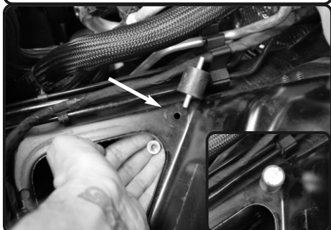
8. Install the vibramount to the hole on frame. Use the M6 nut and secure.
