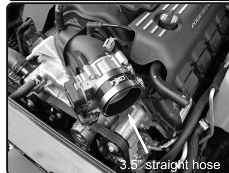
7. Install the 3.5" straight hose to the throttle body. Tighten clamp on throttle body using 8mm nut driver.
