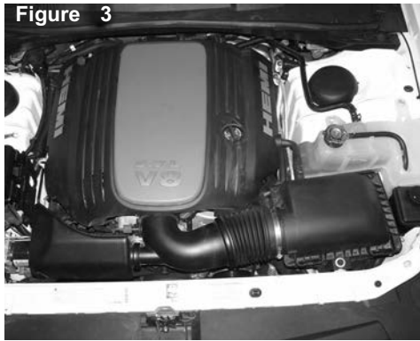
Stock air intake box and air intake duct shown above.
