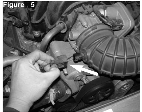
Once the engine cover is removed, disconnect the harness from the air temperature sensor
