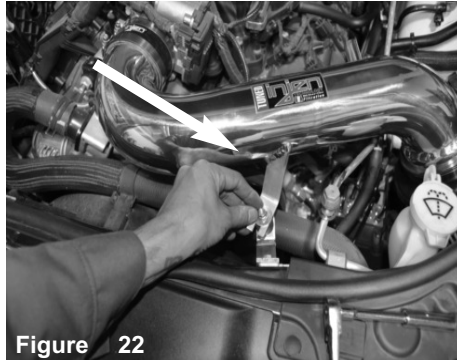
Figure 19 Install the provided grommet to the hole on the intake tube.
