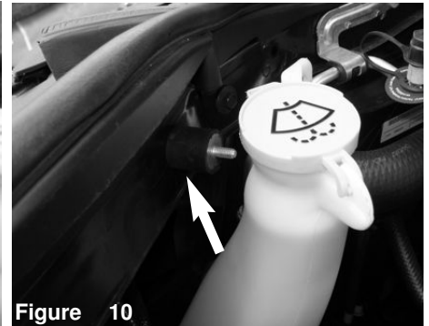
Figure 10 Install the male/male vibra mount secure the back of the vibramount using provided m6 nut.
