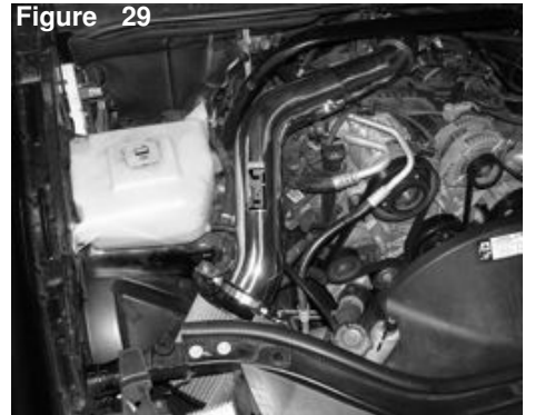
Your Injen intake installation is now complete. Check for any rubbing or any rattling. Tighten all clamps and re-tighten if necessary.
