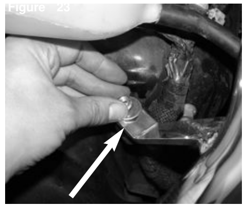
Secure the bracket using M6 nut and washer.
