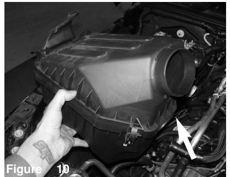
Figure 7 Carefully pull of the intake tube. Note: Temp harness still connected. See next step.
