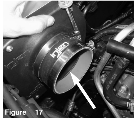
Figure 17 Attach the 3-3/4" straight hose to the powerflow box flange and tighten the clamp using 8mm nut driver.
