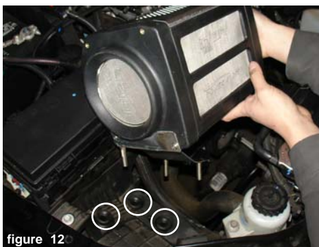
figure 12 Once the bracket has been installed, continue to lower the entire power box in the the engine compartment. The three metal pegs are aligned to the stock grommets and plunged into the grommets.
