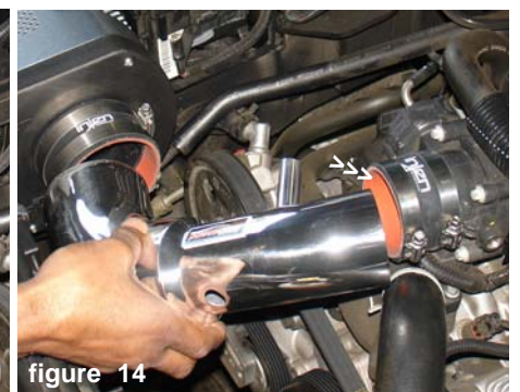
figure 14 The air intake is now lowered into the engine compartment, the upper end is pressed into hose on the throttle body.
