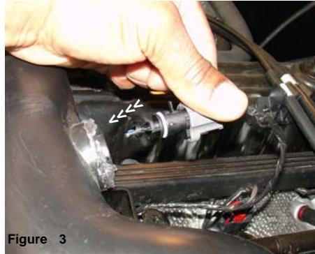
Figure 4 Remove or unhook the clips holding the air box top.
