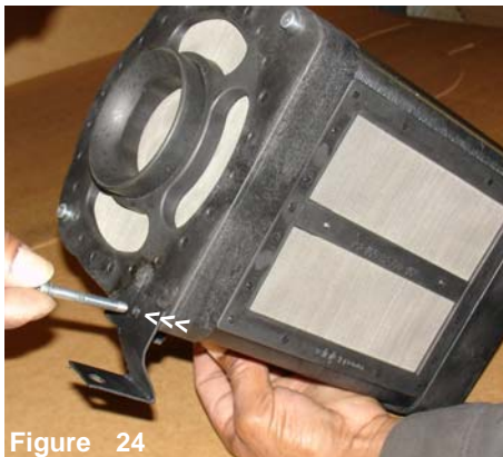
Figure 20 The m6 x 65mm bolt is loosened and removed from the velocity stack base.
