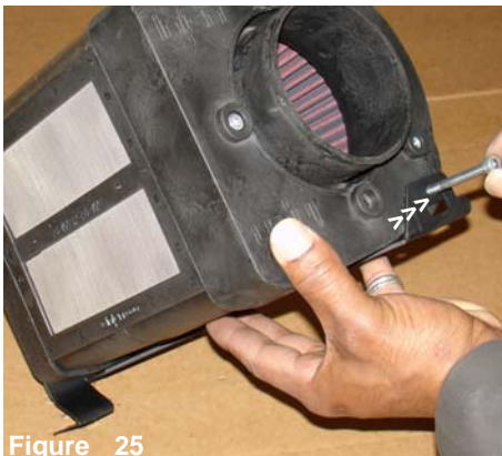
Figure 22 With the rectangular screen facing you, position the bracket as shown above. The power box will slip into the side saddles.
