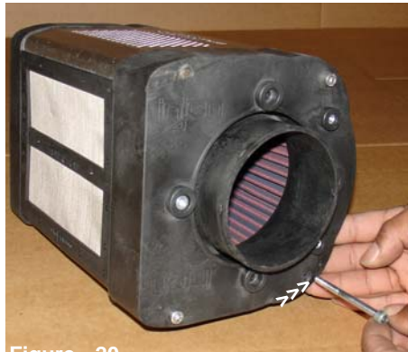
Figure 20 The m6 x 65mm bolt is loosened and removed from the velocity stack base.
