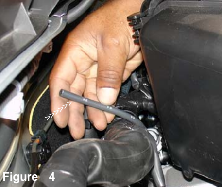
Figure 4 Once the cover has been removed, continue to disconnect the 4mm vacuum line located behind the air box cleaner.
