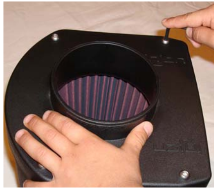
Unbolt the four-m6 x 20mm screws from the velocity stack base located to the center of the base. Now separate the base from the body.
