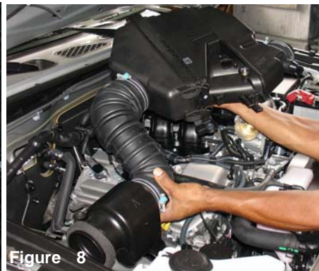
Figure 8 The entire air box cleaner and resonator box is now ready to be removed from the engine compartment.
