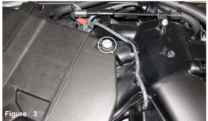
Figure 3 Unbolt the second m6 bolt located on the top of the air box cleaner as shown above. Removing these two bolt shown in figures one and two will allow you to remove the entire air box cleaner. Note: Cover has been removed
