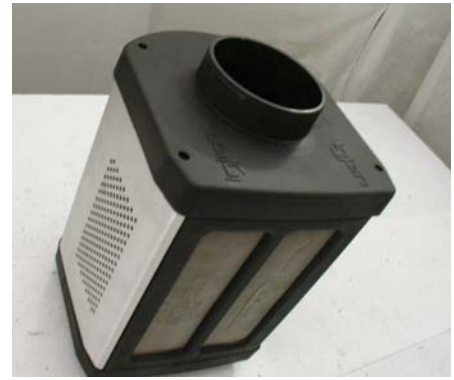
The four m6 x 20mm bolts have been removed from the top of the velocity stack.
