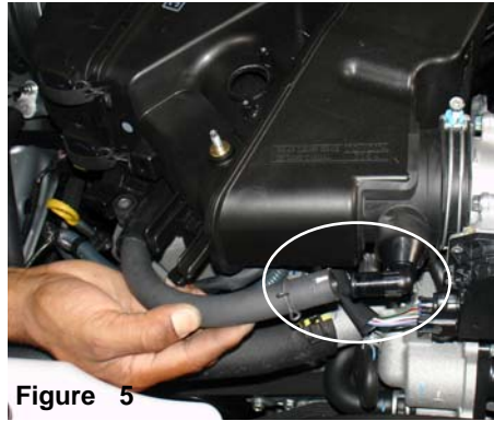
Figure 5 Unplug the crank case breather hose from the air box cleaner port as shown above.
