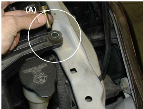
Remove the 6mm bolt located on the cross member. This will allow you to remove the entire air intake box.
