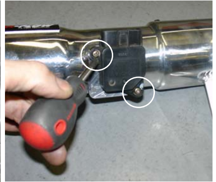
Without pinching the O-ring on the MAF sensor, press the sensor into the flange adapter and use the stock screws to firmly attach the MAF sensor.
