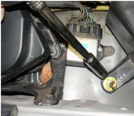
Remove the 6mm bolt by the cruise control box in order to remove the air intake box.
