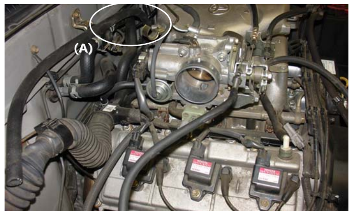
Once you have removed the stock vacuum at the intake port replace it with the 19" 10mm vacuum hose (A).
