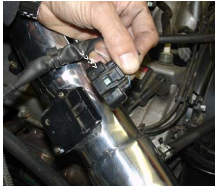
The harness clip is reconnected to the MAF sensor. Press the clip over the sensor until you here it snap in place.
