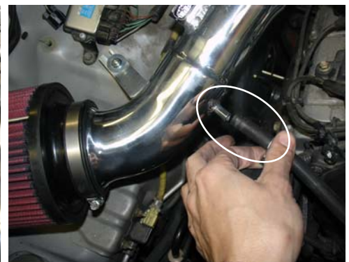
Take the stock 8mm breather hose connected at the crank case port and press it over the 1/2" intake port. Use the stock clamp to secure the hose in place.
