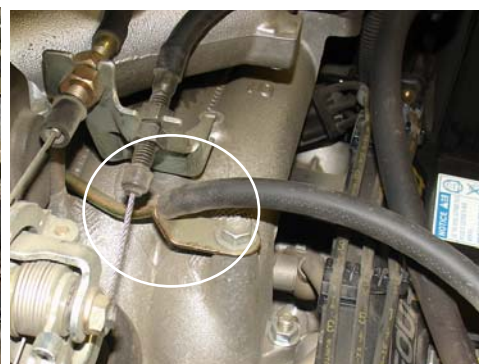
Press the 27" 6mm vacuum hose over the small intake port as shown above. This line will connect to the 3/8" center port nearest to the throttle body.
