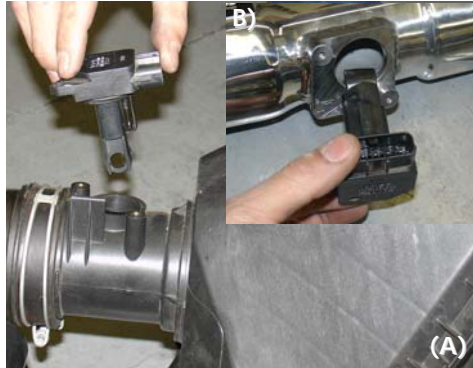
Unscrew the stock screws and remove the mass air flow sensor from the air intake box (A). Slowly, insert the mass air flow sensor into the machined MAF sensor flange as shown above (B).
