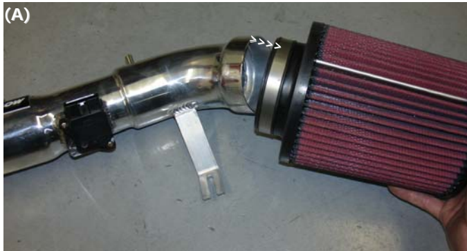
Press the 3 1/2" filter neck over the intake as shown above. Once the filter has been properly placed continue to tighten the filter neck clamp.
