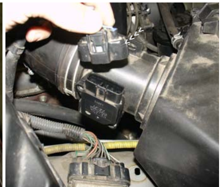
Disconnect the harness clip connected to the air mass sensor.
