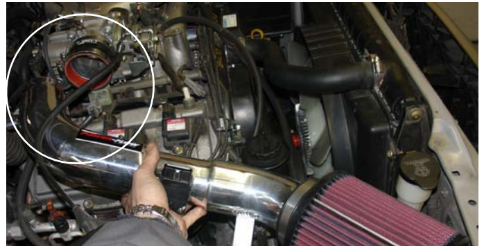
Lower the entire intake assembly into the engine compartment and press the top end into the 2 3/4" straight hose.
