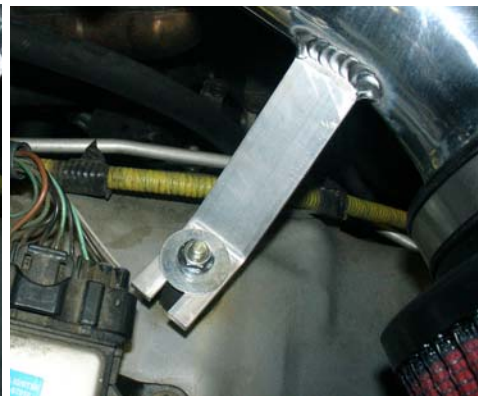
The m6 flange nut and fender washer are used to secure the intake bracket to the vibra-mount stud.
