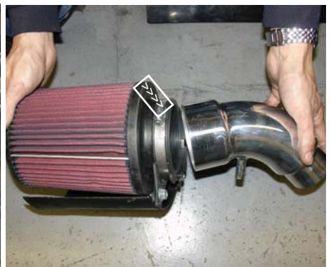
Press the 3 1/2" filter neck over the secondary intake as shown above. Once the intake has butted up against the filter neck stop continue to tighten the clamp. The Power-heat shield shown on the filter is an accessory not included in this kit.
