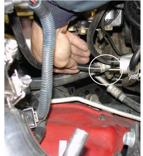
The other end of the 18" -6mm vacuum hose is pressed over the power-steering switch port as shown above.
