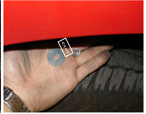
Reach underneath the wheel well and use the m6 flange nut and washer to secure the vibra-mount in place.
