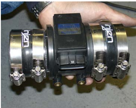
The mass air flow sensor is now assembled and ready for installation.
