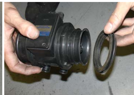
The sealing grommet has been removed and set aside. This grommet will not be needed to complete the installation.
