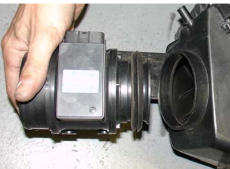
Once the two bolts have removed continue to pull the air mass sensor out from the air intake box as shown above.
