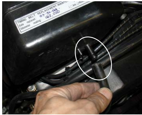
Remove the stock 6mm hose located on the side of the air resonator box. This line leads to the charcoal canister port located to the bottom.
