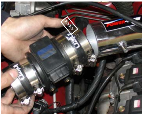
The outlet end of the mass air flow sensor is lined up to the primary intake. Semi-tighten the power-clamp on the intake side just enough to hold the mass air sensor in place.
