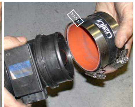
Press the 3" straight hose over the outlet end of the mass air flow sensor. Use two Power-clamps and tighten the clamp on the mass air sensor side.
