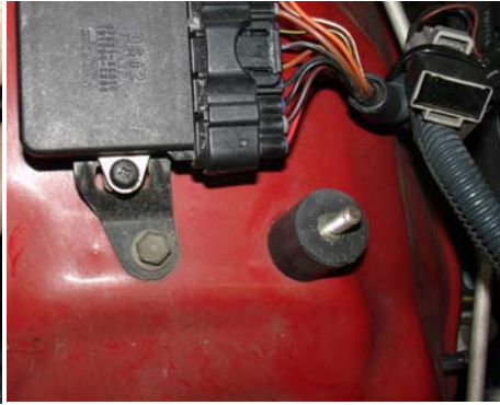
The vibra-mount is now sitting flush with the wheel well fender.
