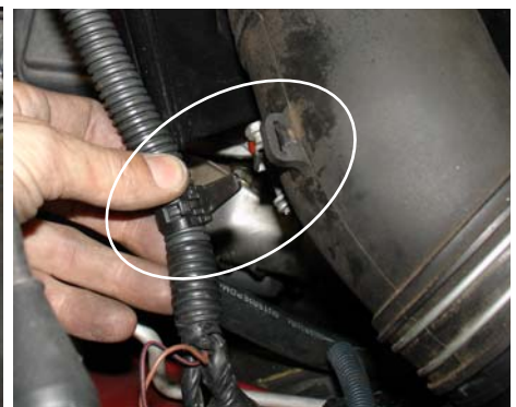
Disconnect the harness clip held on to the lower air intake duct.
