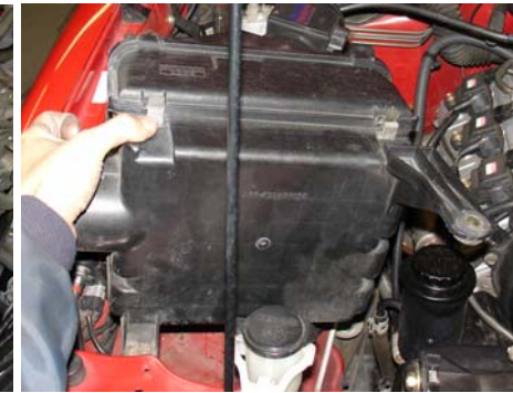
Remove the m6 bolts that secures the air intake box to the wheel well. Once all bolts have been removed continue to remove the entire air intake box from the engine compartment.
