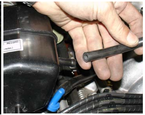
Remove the 6mm stock hose connected to the air intake resonator box. This hose leads to the fuel pressure regulator below the throttle body.
