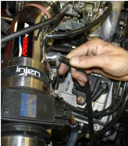
The 18"-6mm vacuum hose is pressed over the second intake port located on the primary intake. The other end lead down to the to Power steering switch port.
