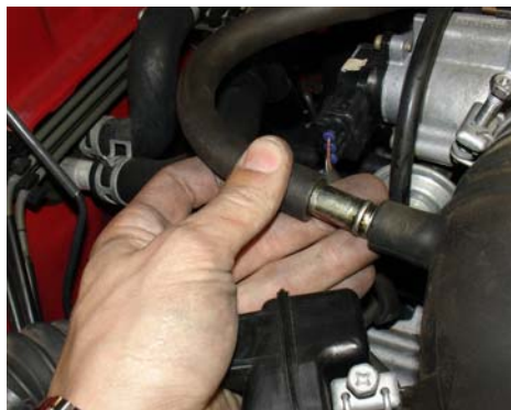
Pull the CC breather line from the air intake duct located by the passenger side firewall. The 13" 10mm vacuum line will be used once the intake has been installed.
