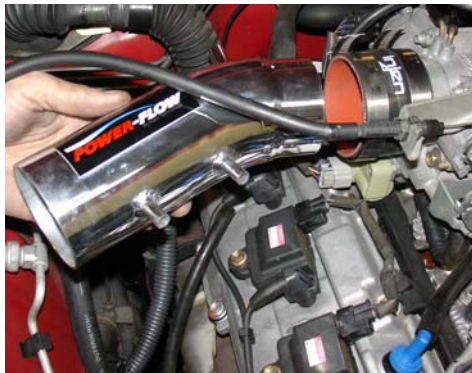
Take the primary intake and press the 2 3/4" end into the straight hose located on the throttle body. Semi-tighten the clamp just enough to hold the primary intake in place.
