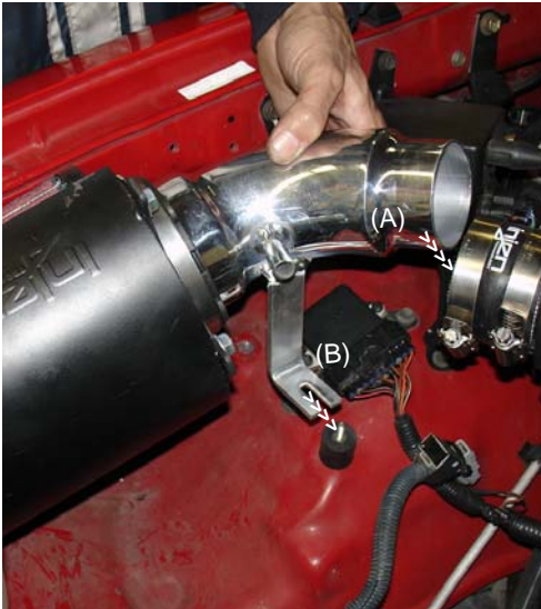
The 2 1/2" end on the secondary intake is lined up to the hose located on the mass air flow sensor (A) . The intake bracket is lined up to the vibra-mount stud (B).
