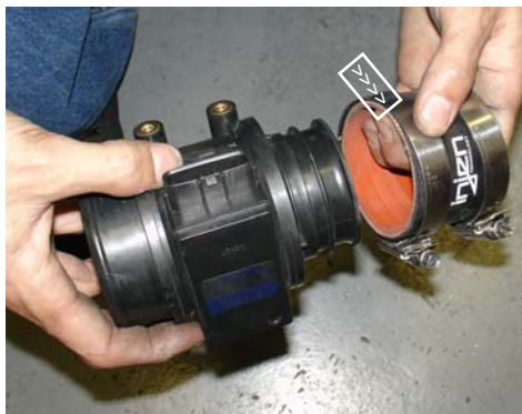
Press the 1 1/2" straight hose over the inlet side of the mass air flow sensor. Use two Power-clamps and tighten the clamp on the mass air flow sensor end.
