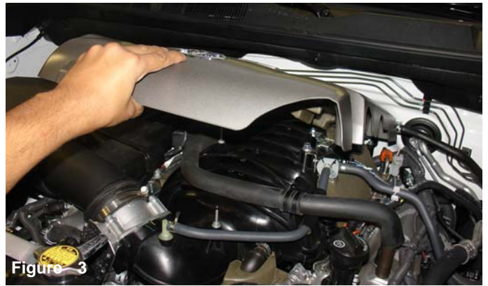
Figure 3 carefully lift up and remove engine cover.
