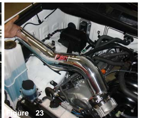
Figure 25 Install intake into vehicle and position.
