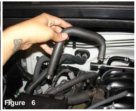
Figure 6 Remove crank case line from vehicle. (will be replaced with provided 15mm hose)
