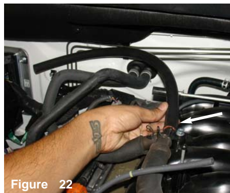
Figure 24 Attach provided 15mm hose to crank case on engine.
