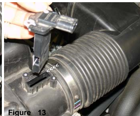
Figure 10 Unscrew the two screws from the mass air flow sensor, shown above.
