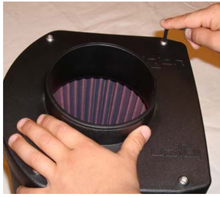
Unbolt the four- m6 x 20mm screws from the velocity stack base located to the center of the base. Now separate the base from the main body.
