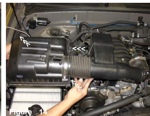
Figure 11 Loosen the hose clamp on the air duct connected to the throttle body.
