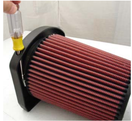
Loosen the clamp on the filter neck in order to separate the filter from the velocity stack.
