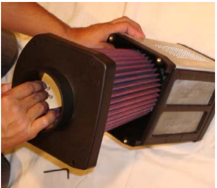
Pull the velocity stack base with the filter that is attached to the velocity stack.
