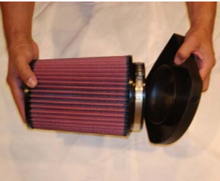
Once you have loosened the filter neck clamp, continue to pull the filter from the velocity stack,
